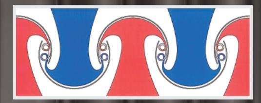
The principle of the cyclone working of the FECON filter. Since 1982
