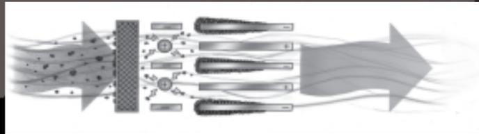
The ionizer consists of charged stainless steel spiked blades spaced between grounded electrodes. The collecting section consists of parallel plates arranged so that each alternate plate is charged while the intermediate plates are electrically grounded.
